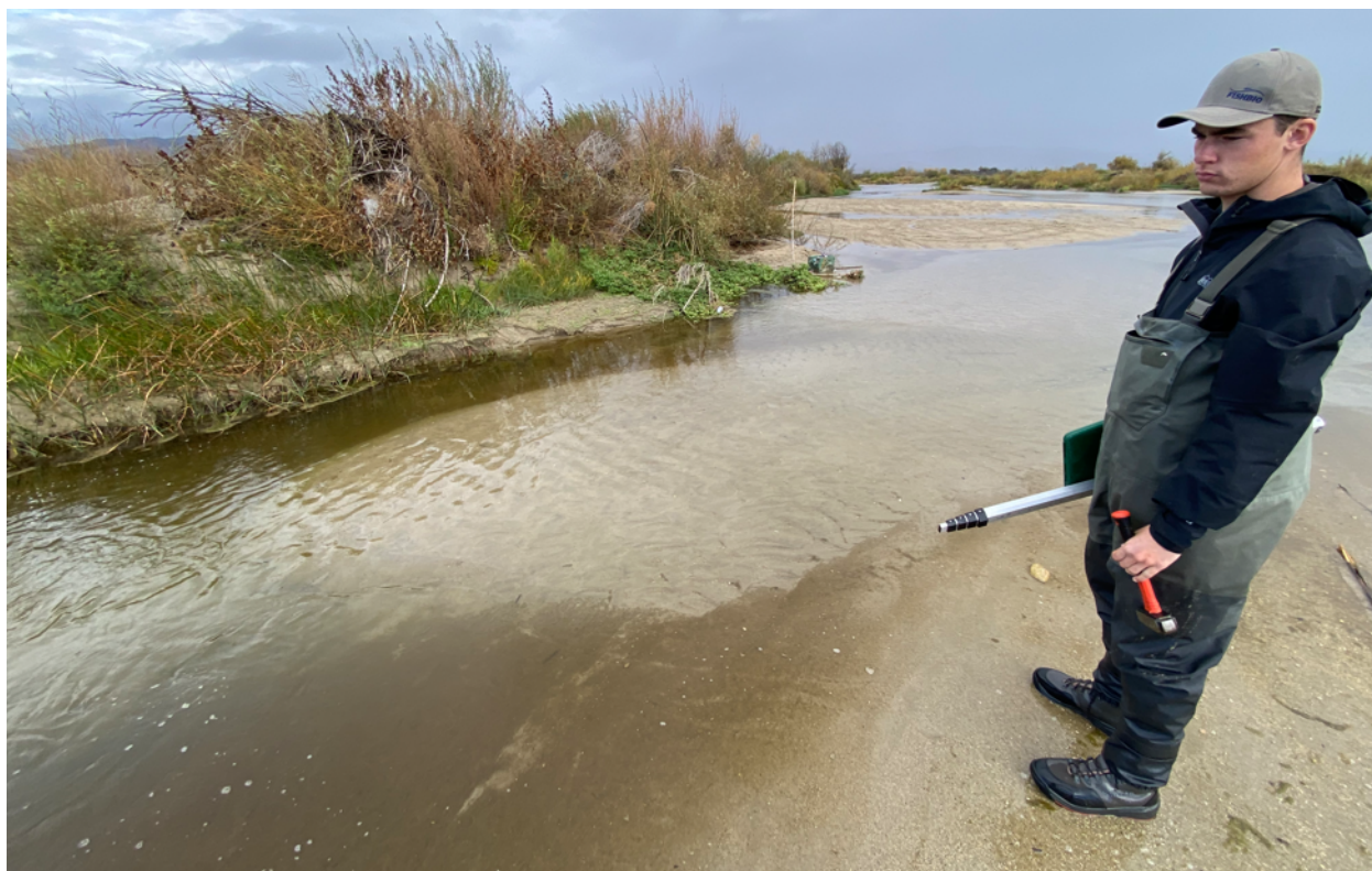
Figure 11. Bed movement of sand into deeper areas of the channel (previously covered in silt) at flows of ~30 cfs in Reach 4 of the Salinas River near Soledad on December 19, 2023.
