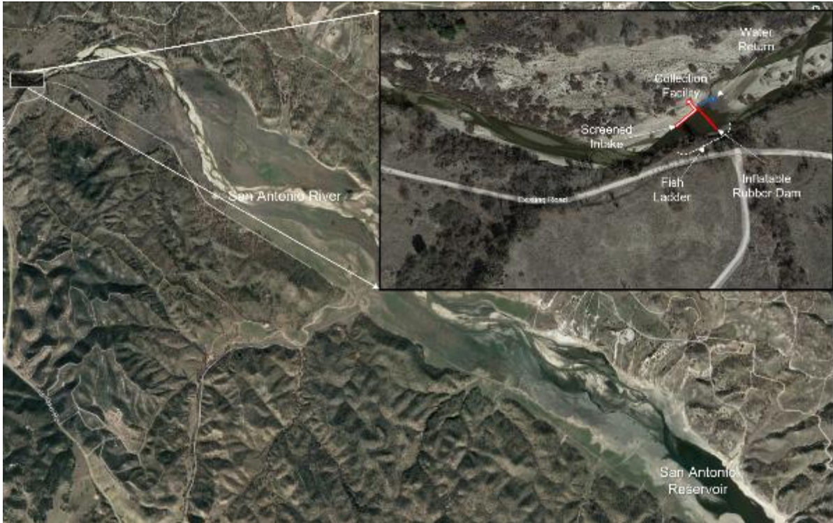
Figure 3-13. Conceptual Example of an In-River Collection System Configuration in the Upper San Antonio River near San Antonio Reservoir
