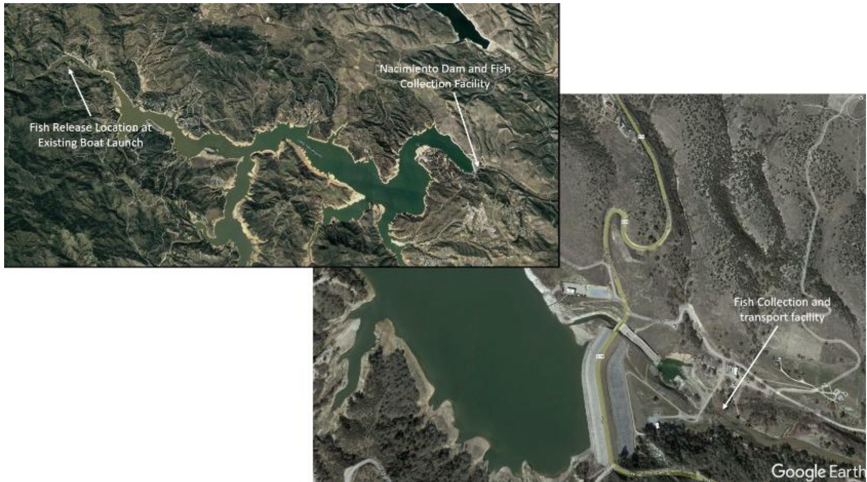
Figure 3-4. Trap-and-Haul Operational Configuration with the Fish Collection Facility at the Base of Nacimiento Dam and the Release Location at the Upper End of the Reservoir at an Existing Boat Launch near Asbury Creek.
