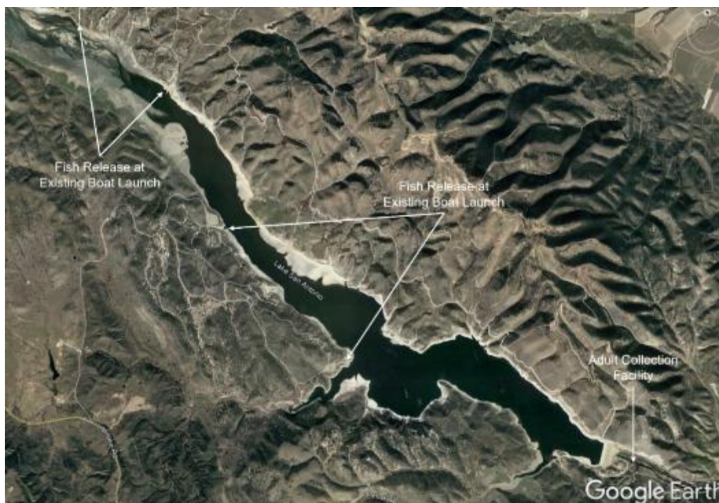
Figure 3-5. Trap-and-Haul Operational Configuration with the Fish Collection Facility at the base of San Antonio Dam with Release Locations at Existing Boat Launches along the Reservoir and Upper San Antonio River
