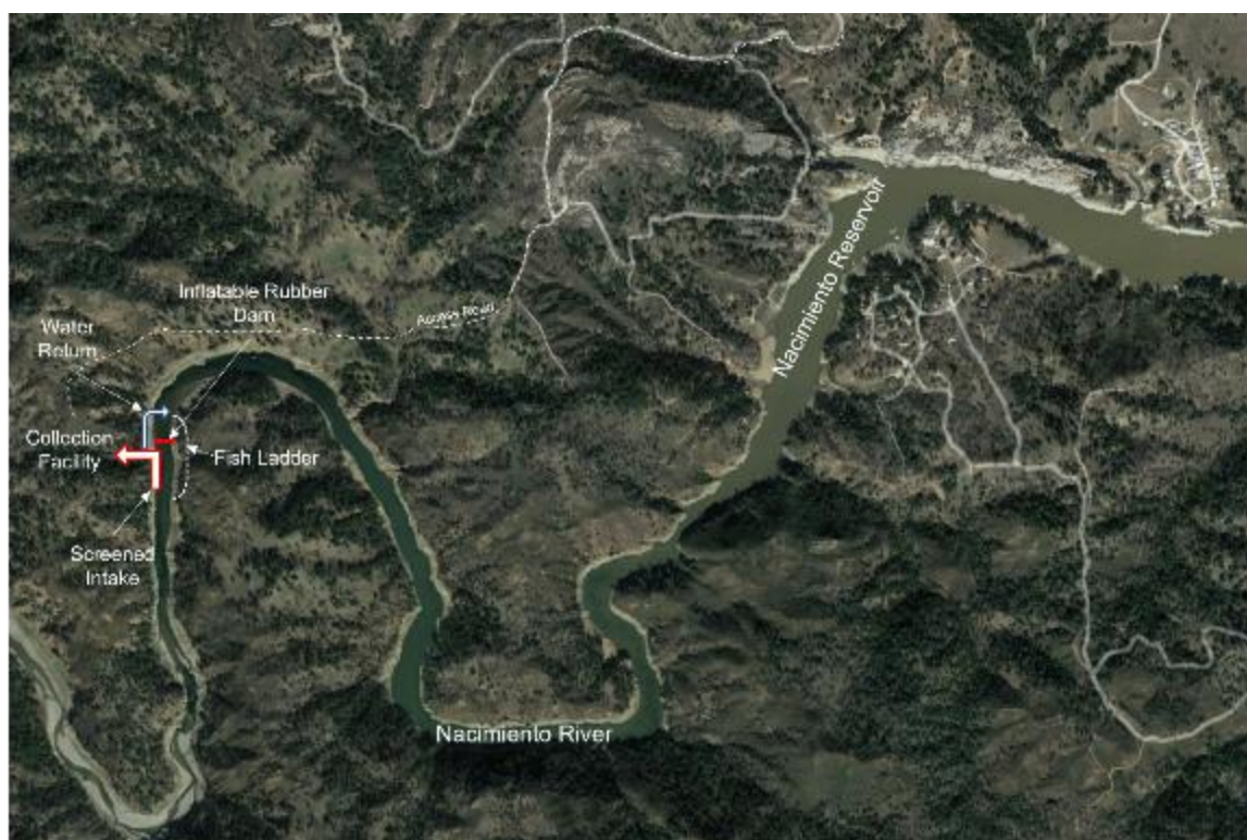
Figure 3-10. Conceptual Example of an In-River Collection System Configuration in the Upper Nacimiento River near Nacimiento Reservoir
