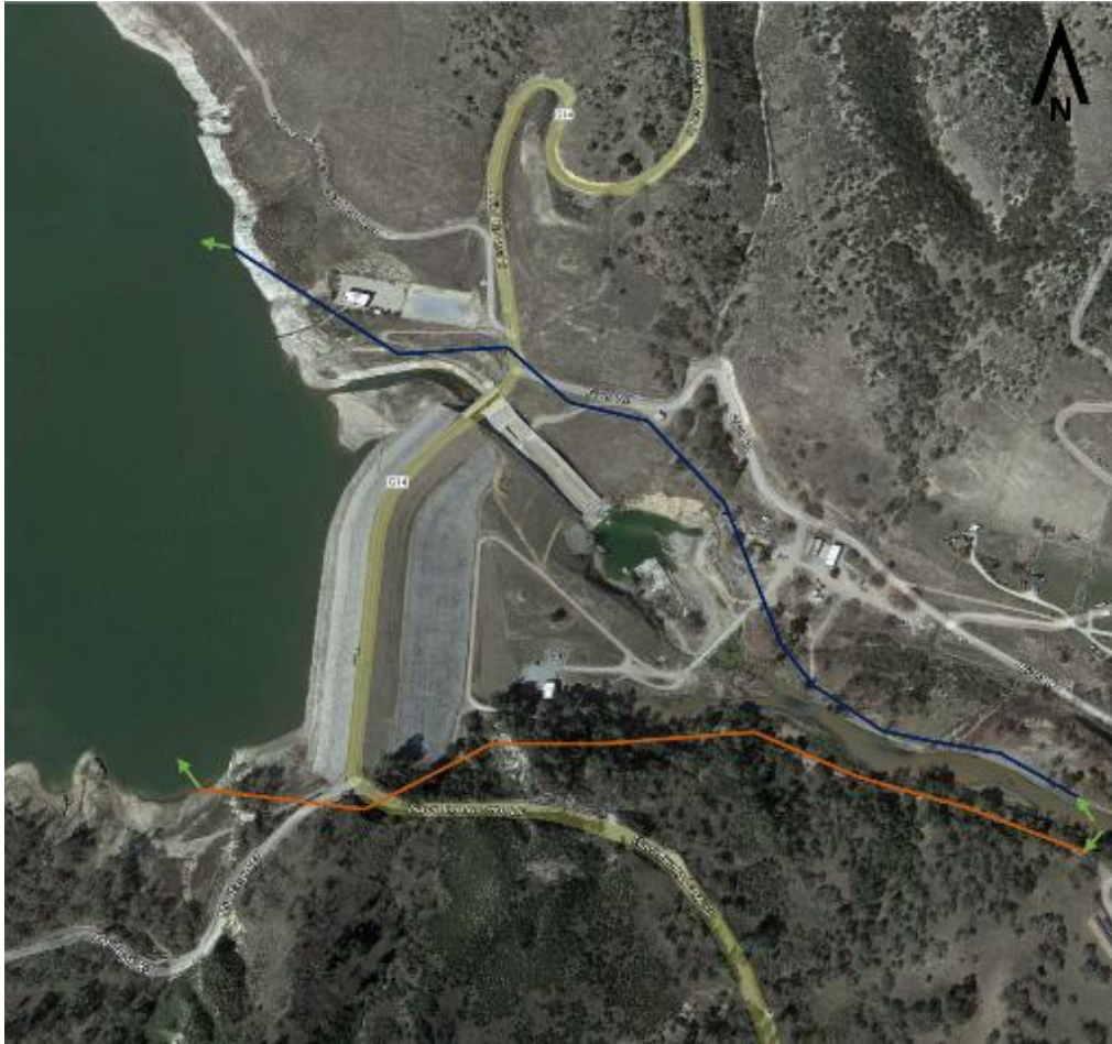
Figure 3-1. Example of fish ladder configurations A (blue line) and B (orange line) at Nacimiento Dam
