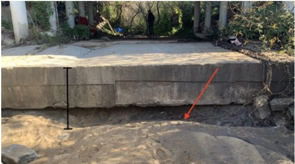
Figure 9. HEB logger site at the time of deployment (January 24, 2020). Arrow indicates the position of the logger, black line indicates height of the barrier, which was 1.22 m above the substrate.
