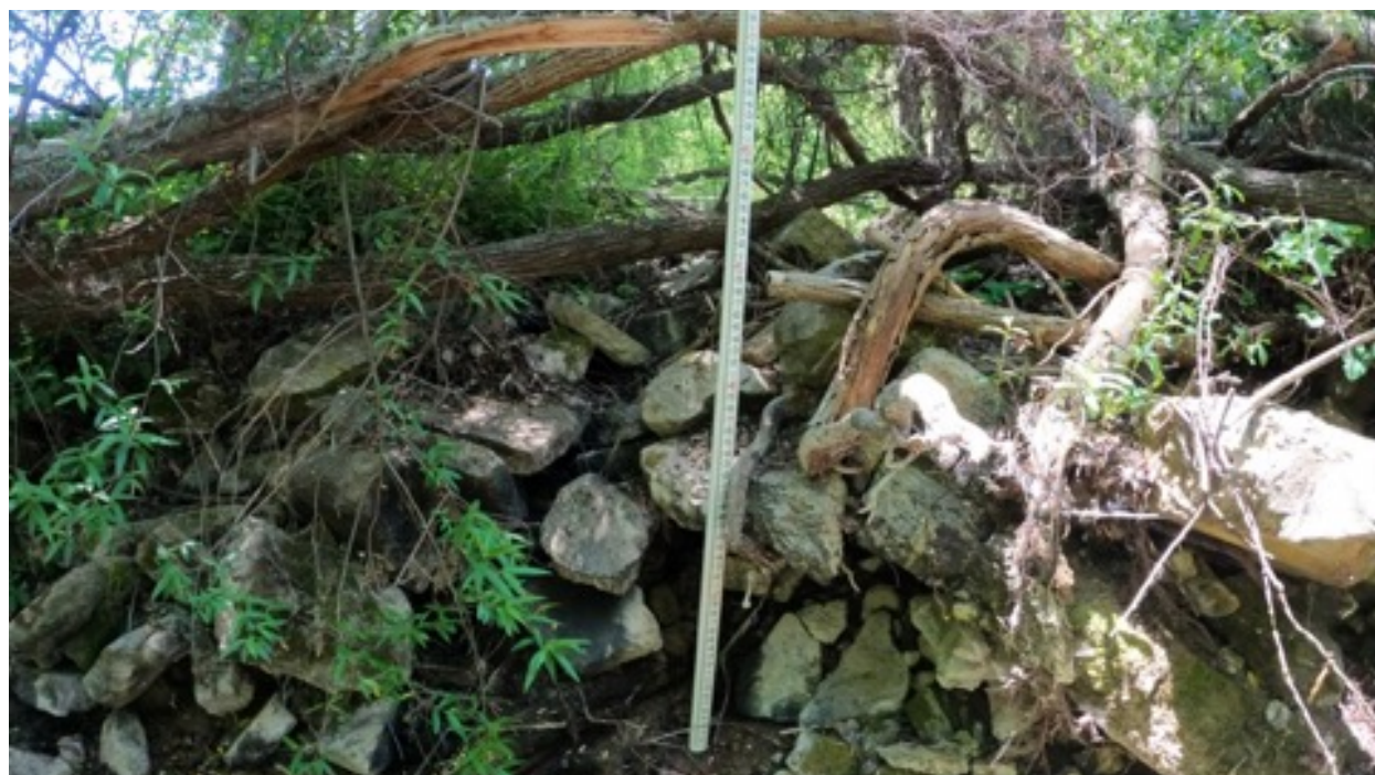
Figure 38. VRB facing upstream. This barrier of concrete, rebar, and woody debris stood approximately 1.68 m tall (5.5. feet). The very shallow puddle visible at the bottom was the furthest upstream observation of water on the Vierra Ranch property.
