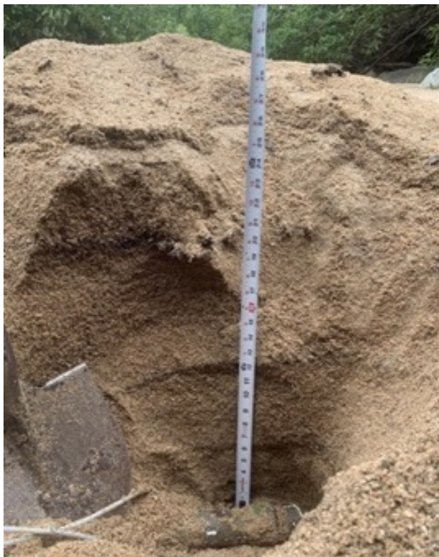
Figure 12. The Hebert Road (HEB) water level logger was buried under approximately 71 cm (~28 inches) of sand sometime during or following the large rain event on April 5. Photo taken April 16, 2020.
